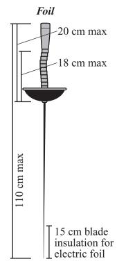
Electrical weapons are used in formal competitions to increase the accuracy of scoring. The weapons are wired. When the weapon blade's button makes contact with the opponent's metallic plastron, electricity is conducted to a body wire. The hit registers on an electrical scoring apparatus: when a touch is scored, a light flashes on a screen on the sidelines. The referee awards touches accordingly.
