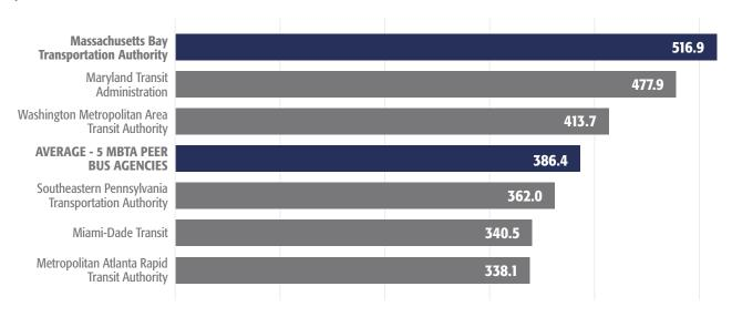
In 2015, the MBTA had the second-highest number of vehicle maintenance labor hours per hour of bus operation among the 25 largest U.S. public transit agencies, as shown in Figure 6. The MBTA had 516.9 bus maintenance labor hours per 1000 hours of bus operations, 41.5 percent higher than the average of 365.2 hours of the 25 largest public transit bus agencies.
